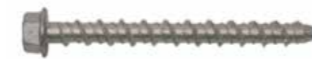
Base tray to foundation example fixing: M6 x 85mm Concrete Bolt with a minimum 1kN pull out. Fixing choice is dependent on substrate.
