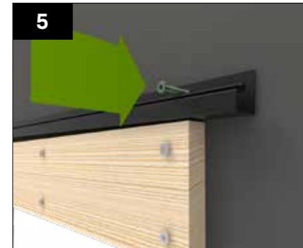
Fit the soaker trim to the wall at a slight angle, giving it a roughly one-degree fall. The battens should terminate above and below this trim.
